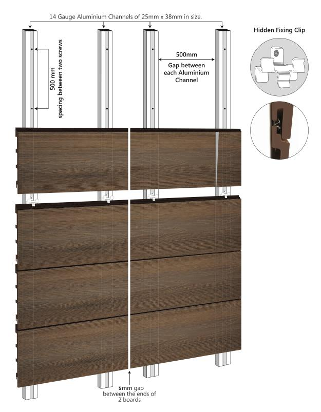
**IMPORTANT**: VENTURA TECHKLAD should always be stored horizontal at site • Installation should go from bottom to top.
